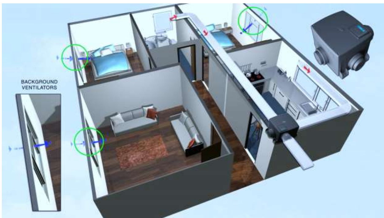
Figure 2: Continuous centralised Mechanical Extract Ventilation drawing fresh air through incorporated background ventilators.
